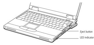
If you have difficulty removing a diskette from the floppy disk drive, remove the floppy disk drive from the multi-purpose bay.
